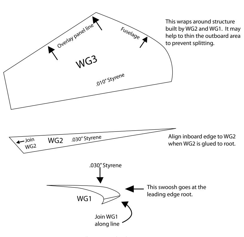
Once all parts are glued, putty any gaps, taking care not to deform WG3. If WG3 get deformed, add very thin putty layers to restore shape.
